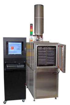
The CD 3045 ovens are controlled by a PLC uploaded from a computer (PC). The main screen of this oven is shown below.
